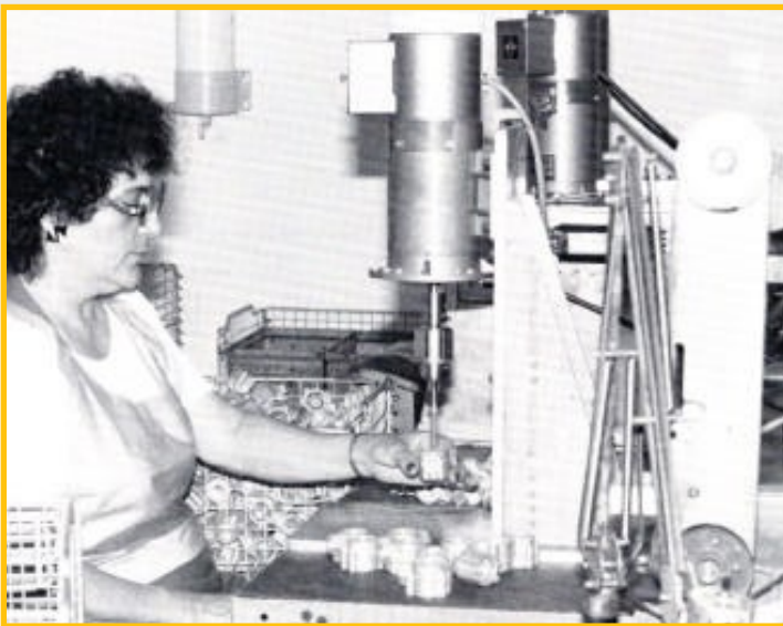
Operator can eliminate inside flashing in seconds. Parts then go to final assembly.
