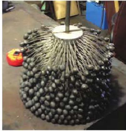
▲ Small, abrasive globules mounted to flexible filaments are the key to how the Flex-Hone works. It is available in many sizes and abrasive types and grits.
