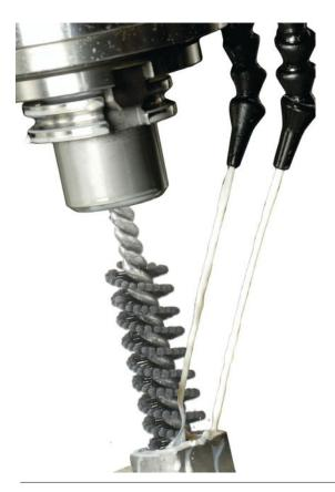
According to Brush Research Manufacturing, the impact of abrasive tools is negligible because filtration systems are already required to remove particulate from the coolant generated during the machining process itself.
