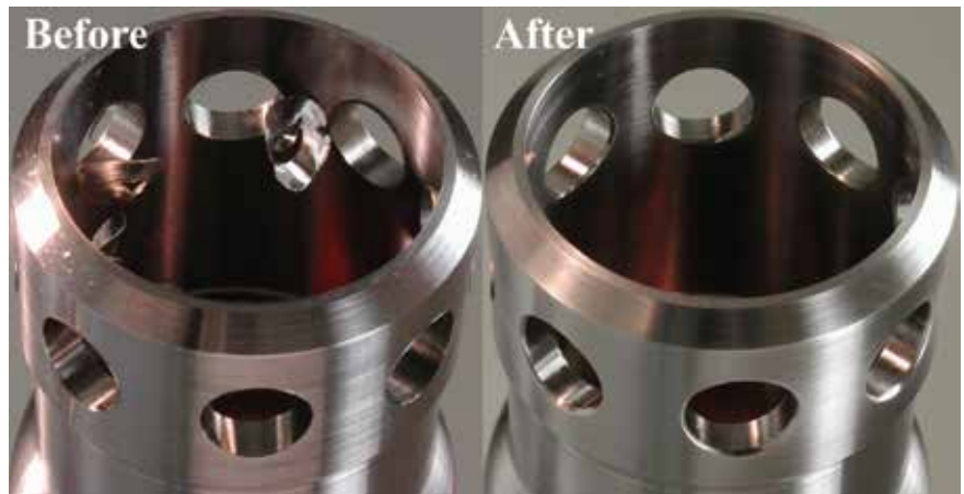
Cross-hole deburring before and after.
