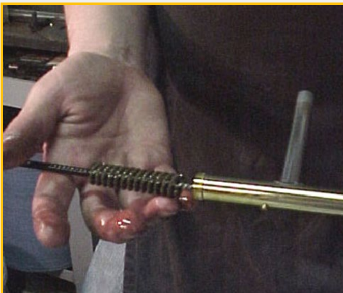
An upclose view of the Flex-Hone®. The Flex-Hone cleans and polishes the inside of the tube.
